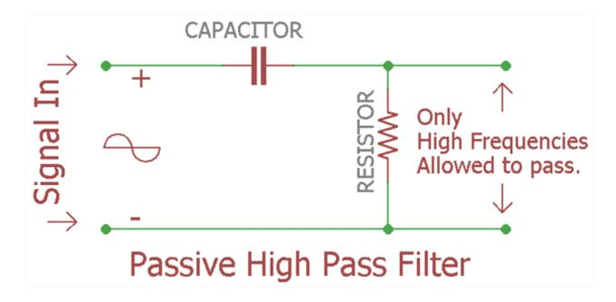
After going through the capacitor, the electrical signal passes through a resistor. Resistors are made of varying materials that have a specific controlled level of resistance to the flow of the electrical current. This could come in the form of carbon powders to metal films. In a high pass filter, the resistor is often used in series with the capacitor to form a voltage divider, cutting off any lower frequencies that were missed by the capacitor.
