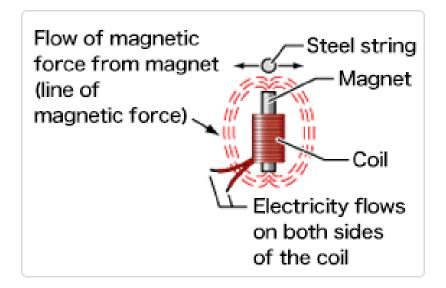
This disturbance is what causes an electrical current to form the coil around the pole pieces. But why does a disturbance in the magnetic field cause an electrical current? The answer lies in Faraday's law of electromagnetic induction.
