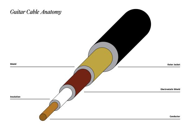
The conductive wire carries the electrical signal from the guitar to the amplifier. The insulating material prevents interference in the signal when traveling from guitar to amp. The electrostatic shield discharges static electricity to prevent the buildup of static charges that cause damage in circuits. All these components are encased in an outer jacket.
