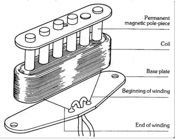
There are two basic types of pickups with a similar anatomy used in the common electric guitar, single coil and humbucker pickups. Both types fulfill the same purpose, but are constructed slightly differently.
