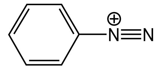
Diazo is typically mixed with polyvinyl alcohol (PVA) and polyvinyl acetate (PVAC). When exposed to UV rays, the diazo undergoes a photochemical reaction, crosslinking the polymers into a solid, insoluble stencil. However, the areas that remain underexposed have not undergone this reaction and remain in a soluble, liquid form. When the screen is washed off with water, the uncoupled polymers dissolve, while the
